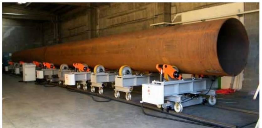
ROLLS SUPPORT WITH HEIGHT ADJUSTMENT FOR PIPES ALIGNMENT
