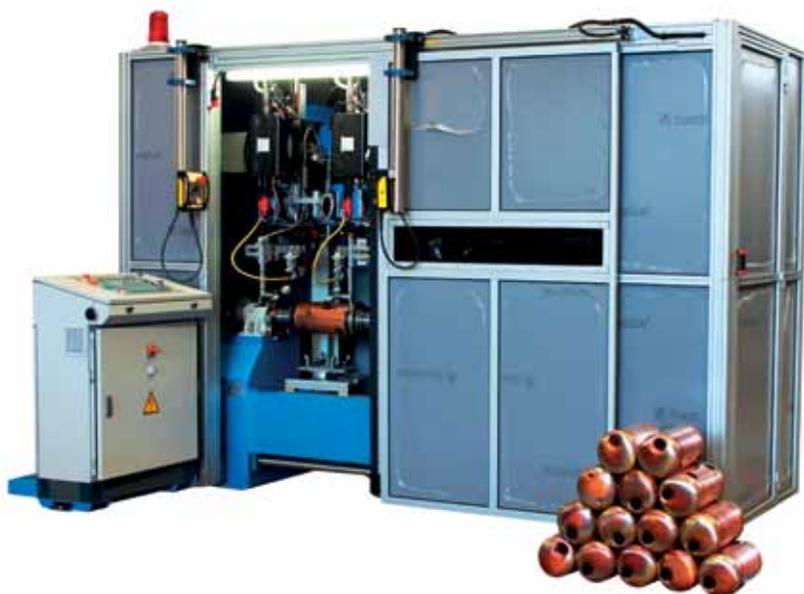
Automatic lathe for the production of tanks for professional coffee machines. Includes double TIG station with cold wire feeder, intelligent tracking system. This machine is equipped by a touch screen control board with PLC to manage all the functions of the system, welding parameters included. Similar solutions are available for a lot of circumferential weldings, also with loading station and automatic discharge.
