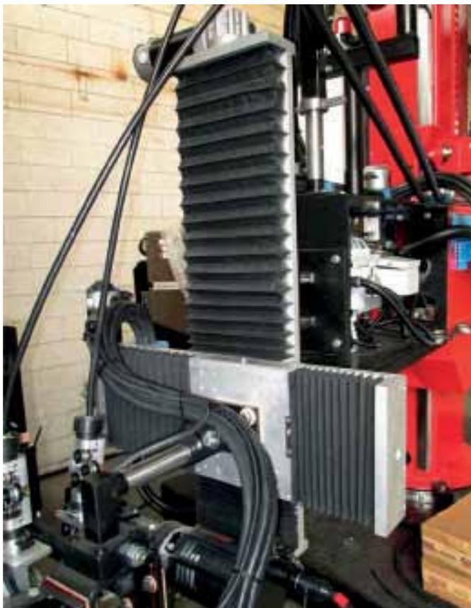
The picture shows a typical X-Y crossed slides system, assembled on a C&B head for SAW procedure.
