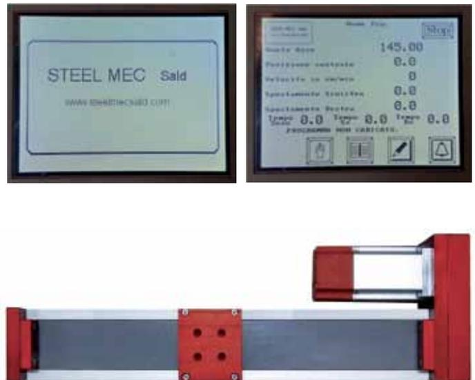
The RED linear OSCILLATOR model shows the best device in this field. Its axle is motorized and is complete of bushless motor with resolver which act a ball recirculating rolled screw connected to the trolley holder torch. The control console is full of touch screen 5,7" panel which allows to manage all the following process variables:
